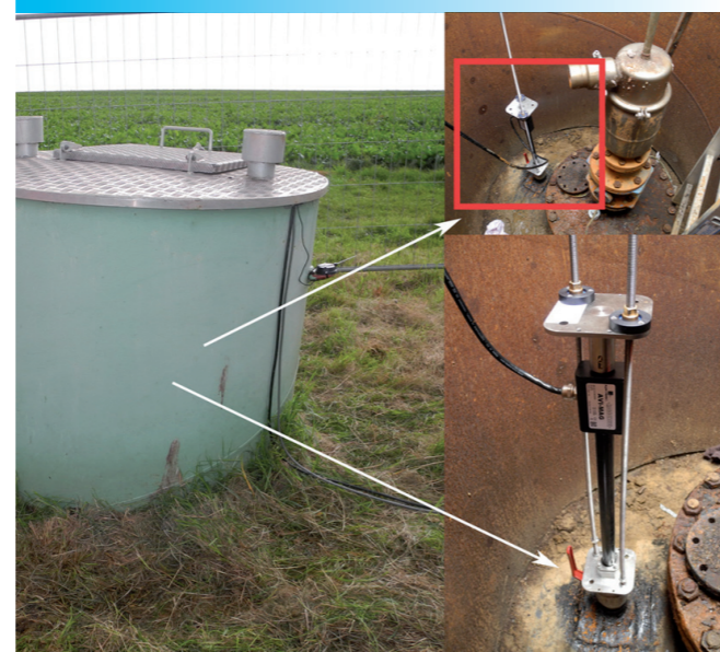
Electrodes repartition on equal areas
